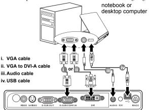
Many notebooks do not turn on their external video ports when connected to a projector. Usually a key combo like FN + F3 or CRT/LCD key turns the external display on/off. Locate a function key labeled CRT/LCD or a function key with a monitor symbol on the notebook. Press FN and the labeled function key simultaneously. Refer to your notebook's documentation to find your notebook's key combination.
